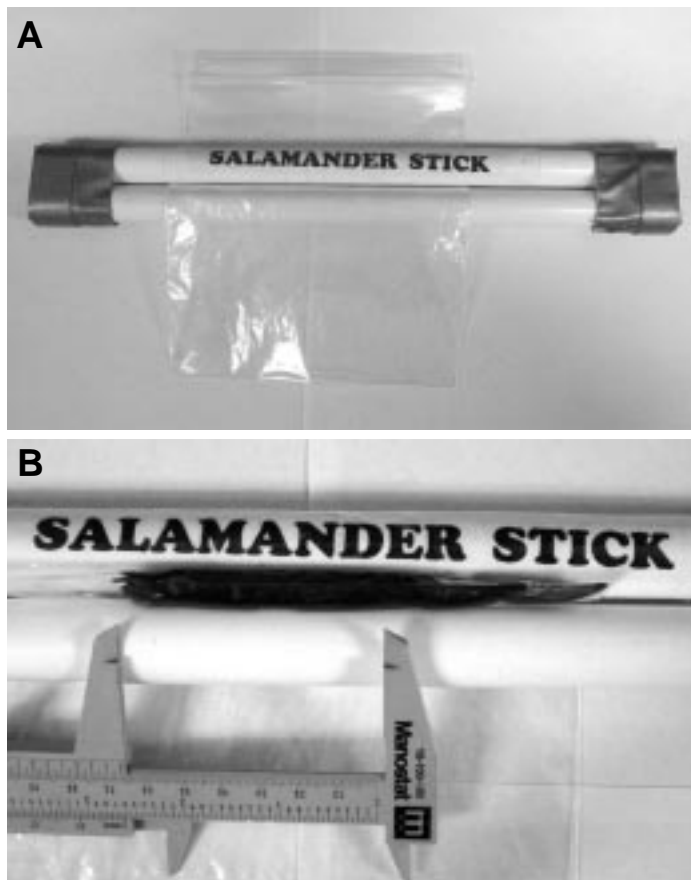
FIG. 1. The Salamander Stick, a device for obtaining precise and accurate measurements of salamander snout–vent length. A) The device shown with a plastic bag passing through the slit between the two polyvinyl chloride (PVC) pieces. B) The lateral view of an adult Smallmouth Salamander ( Ambystoma texanum ) immobilized in the device.
